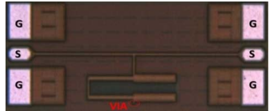
Fig. 6. The chip photo of the fabricated resonator.
